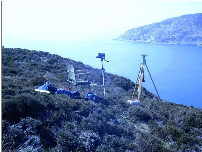
Figure 11. The set-up at the viewpoint, showing the scope, mount and theodolite. The view looks northeast with the southwest tip of Scarba in the background.
